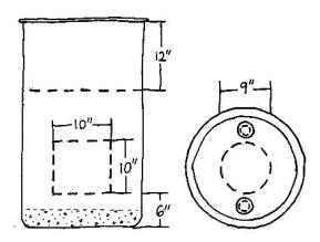
JTEP 1 Using a jigsaw, cut the barrel in two @ 12" from the top of the barrel. Also, cut a 9" diameter round hole in the top and a 10"x10" square hole on the side of the barrel @ 6" above the bottom of the barrel. Following the instructions on the package, Mix the bag of concrete with water and fill the bottom of the barrel with it. Use a trowel to level and smooth out the surface of the concrete.
